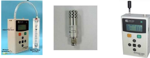
Figure 4: Monitoring PM instrument and its calibrator.
