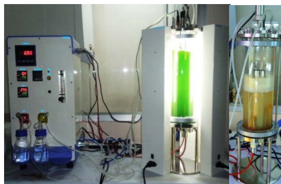
Figure 2: Haematococcus pluvialis cultivation and red stage (Aplanospore) in Photobioreactor
