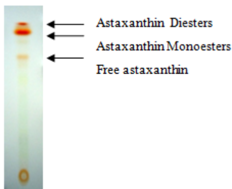
Figure 3: TLC sheet showing Astaxanthin and their derivatives
