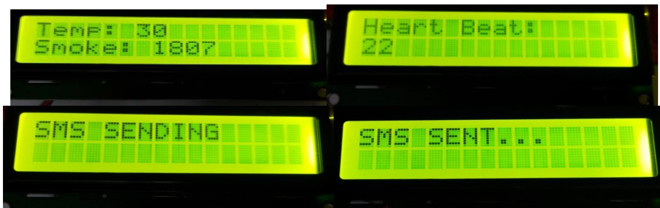
Figure 4: Output (patient information) shown in LCD
