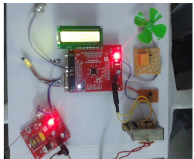
Figure 2: The Microcontroller Lpc 2148 using experimental kit
