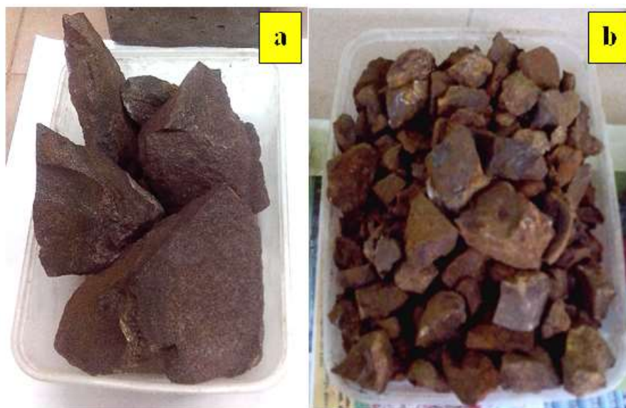
Figure 3: Optical graphs (a) show the hematite rocks before crushing (b) after being crushed to suitable sizes.
