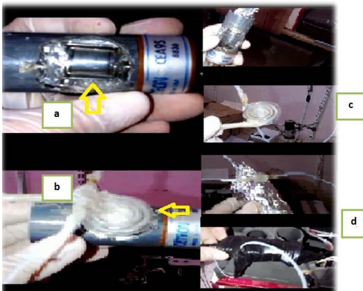
Figure 7a, b: The PMT was attached directly to the home-made glass flow coil, c glass flow, d covered with sheet of aluminum foil and black chamber of PMT
