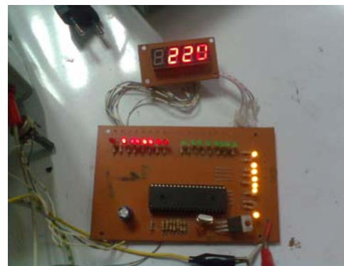
Figure 6: Digital voltmeter with 7-segment display (in the lab).
