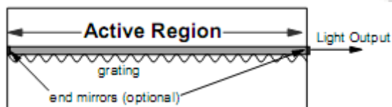
Figure 3.2: Schematic diagram of DFB Laser [1]
