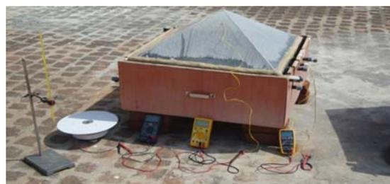
Figure 1: Pyramid Type solar still
