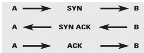
Figure 5: A Normal TCP Connection Request from A to B
