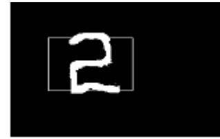
Figure 10: To locate the object position(After masking process)
