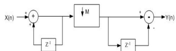
Figure 2: Implementation of RRS using down sampler
