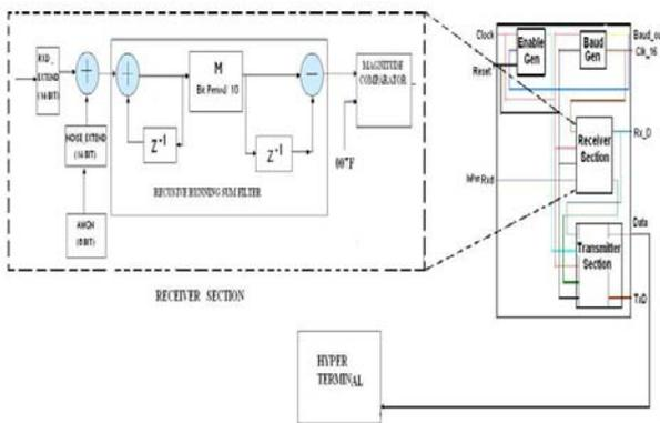
Figure 4: The UART block diagram
