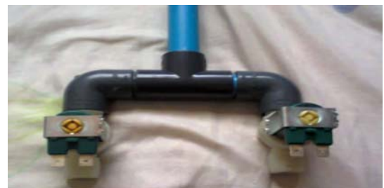
Figure 8: Fabricated solenoid valves
