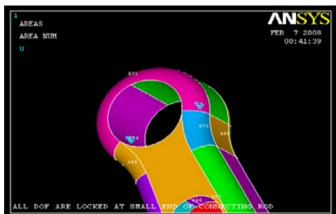
Figure 4: Applying pressures to the connecting rod at the big end and small end.
