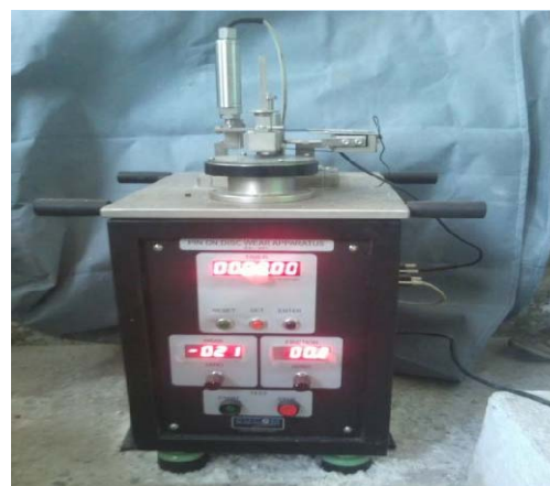
Figure 1: Pin on Disk apparatus
