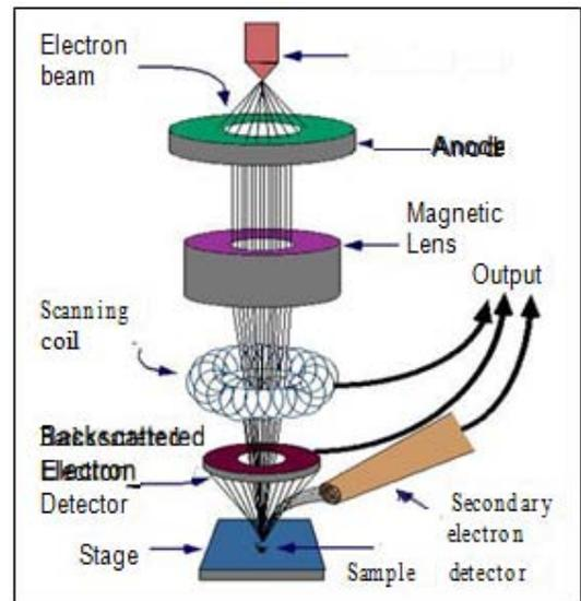
Figure 1: Simplified Schematic of SEM/SEBL
