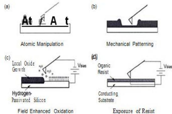
Figure 2: Nano patterning methods using SPL
