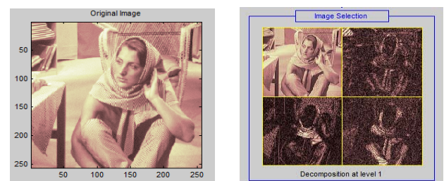
Figure 3: (a) Original Barb image and (b) One level DWT transform
