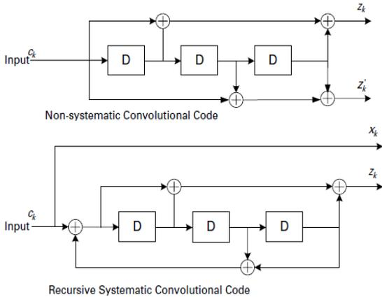
Figure 2: Conventional convolutional encoder and equivalent RSC encoder [3]
