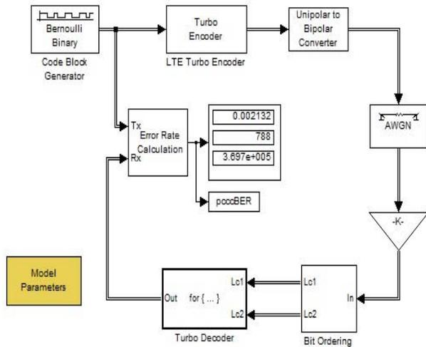
Figure 5: Parallel Concatenated Convolutional coding: Turbo codes [6]
