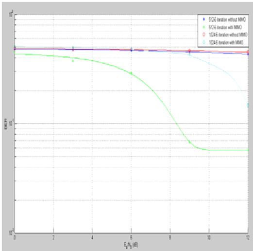
**Figure 9:** Plot of BER vs *E<sub>b</sub>/N<sub>0</sub>* PCCC with and without MIMO channel
