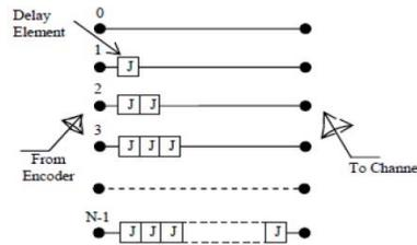
Figure 4: Convolution Interleaver
