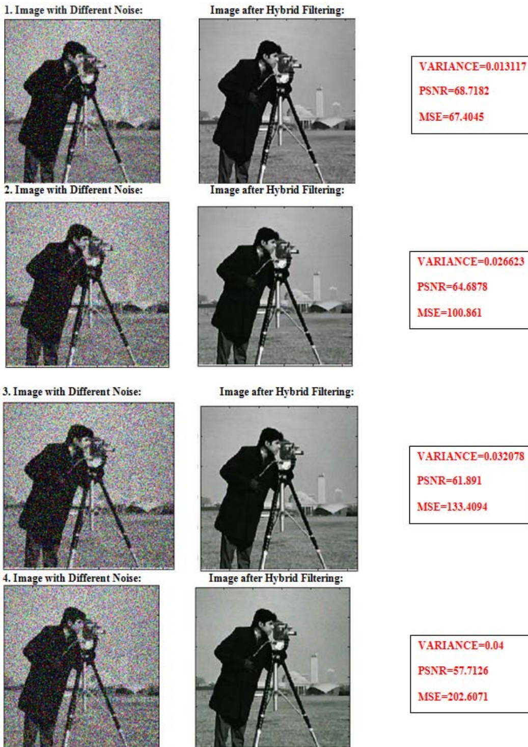
Figure 1.13: Shows the images corrupted with different noise variance are filtered with mixed mode filtering and describe the PSNR and MSE
