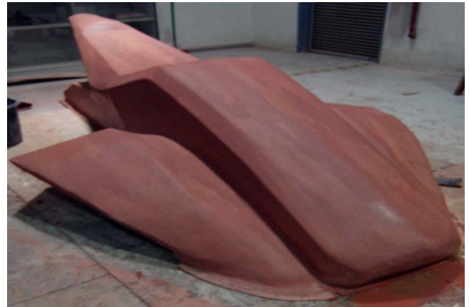
Figure 7: Surface finishing of the Bodywork
