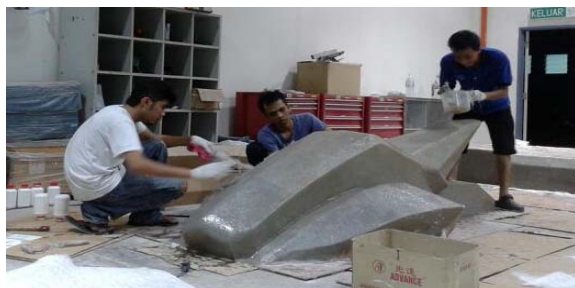
Figure 6: Hand layup technique
