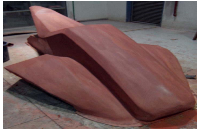
Figure 7: Surface finishing of the Bodywork
