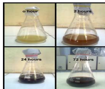
Figure 1: periodic colour change of the reaction mixture (fenugreek seed extract+ 1mM AgNO 3 )
