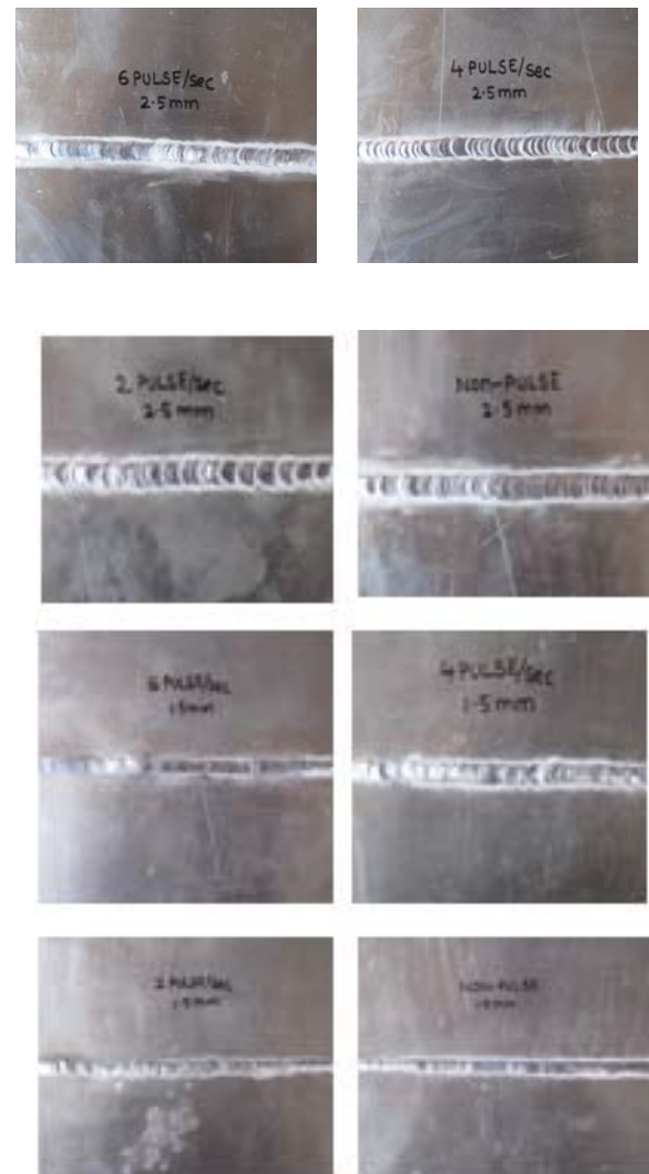
Figure 7. Welded Plates of Aluminium Alloy 5052
