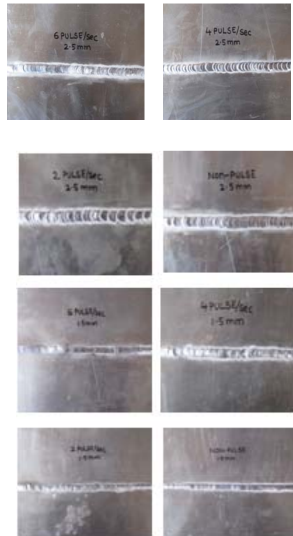
Figure 7. Welded Plates of Aluminium Alloy 5052
