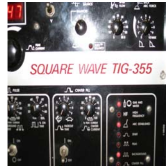
Figure 5. AC/DC Pulse Panel
