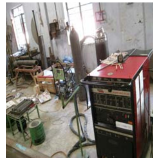
Figure 6: Lincoln Electrical square wave TIG 355 GTAW
