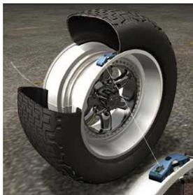
Figure 4: Tier Pressure Sensor
