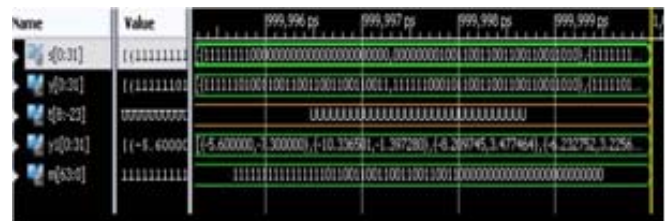
Figure 7: Simulation results of the 32-point FFT
