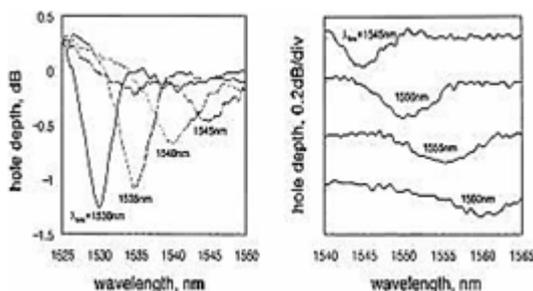
**Figure 3.** Spectral Hole Depths versus Wavelength
