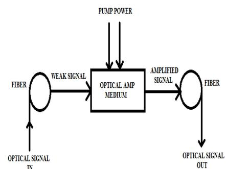
**Figure 1.** General Representation of an Optical Amplifier
