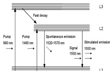
Figure 2. Energy levels of Erbium ions in EDFA [6]
