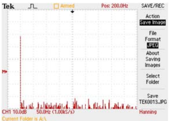
Figure 16: Harmonics without filter
