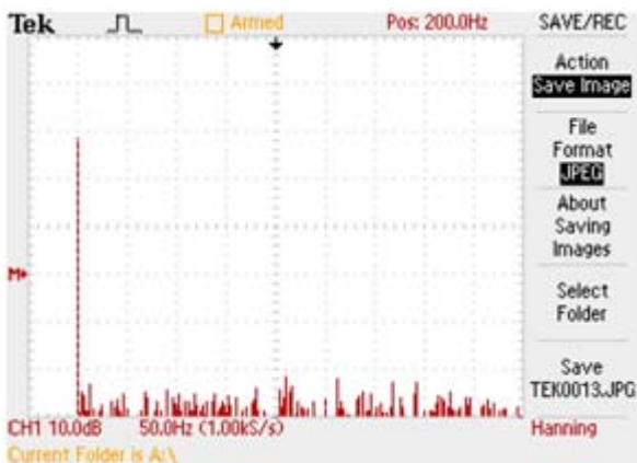
Figure 16: Harmonics without filter
