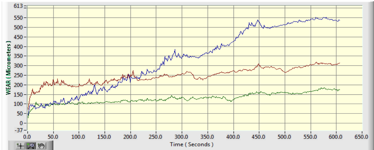
Figure 3: Al6063+0% Al 2 O 3 , Al6063+4% Al 2 O 3 , Al6063+8% Al 2 O 3 at 3.5m/s sliding velocity
