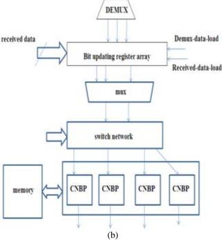
(b) Block parallel layered decoder architecture.
