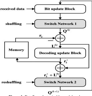
Figure 1: Dataflow of a typical layered decoder
