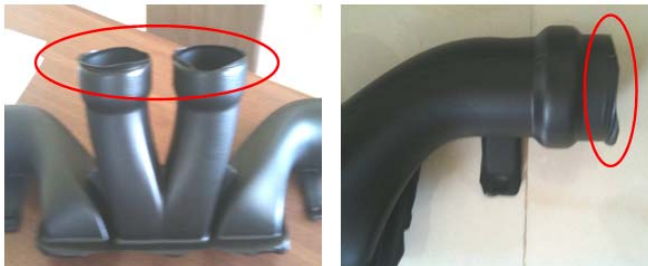
Figure 1: Defects in Air duct
