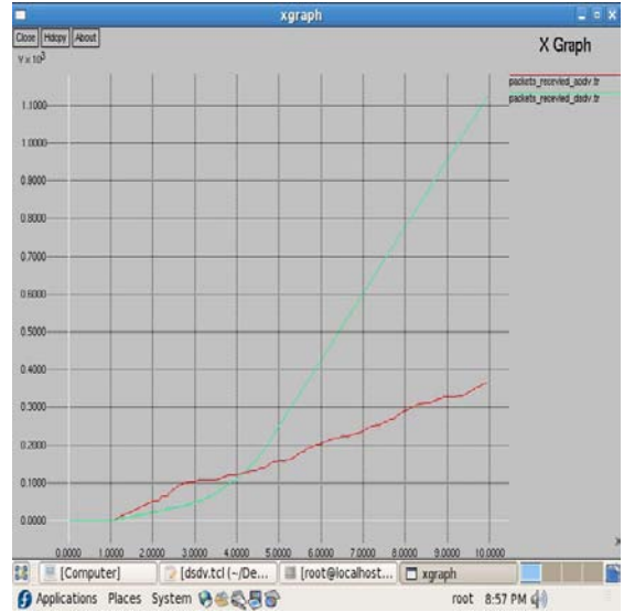
Figure 11: Comparing received packets of AODV and DSDV
