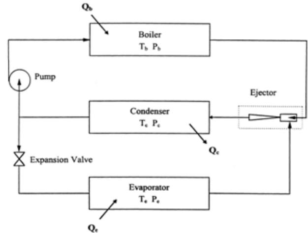
**Figure 1:** Schematic diagram of Ejector refrigeration system
