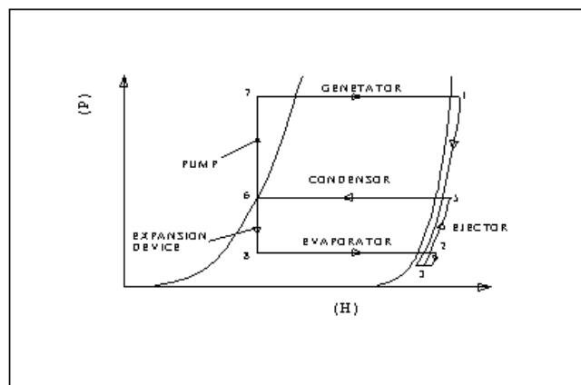
**Figure 4:** Ejector refrigeration system on P-H diagram
