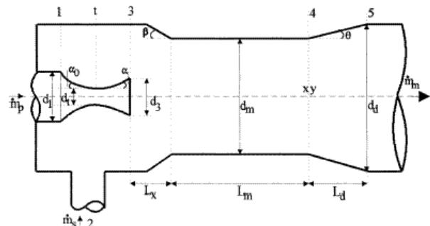
**Figure 2:** Schematic diagram of Ejector showing various sections
