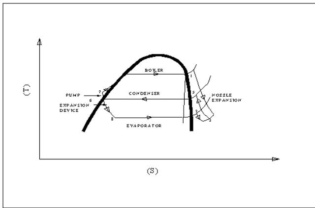
**Figure 3:** Ejector refrigeration system on T-S diagram
