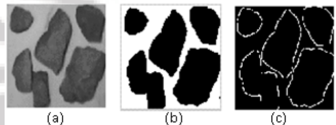
Figure 1: (a) Gray level image, (b) Thresholding with a global value of 120, (c) Edges detected using Sobel masks
