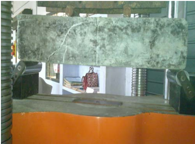
Figure 5: Crack Pattern of beam obtained in two points loading
