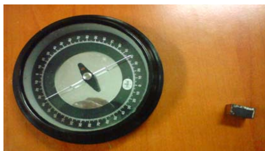
Figure 2: Magnet placed near a magnetometer
