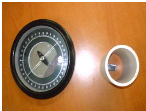
Figure 8: Magnet housed in a PVC cylinder
