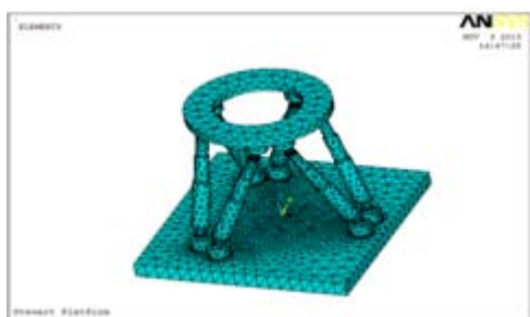
Figure 4: Model and Meshing
