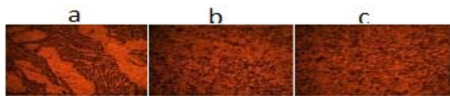
Figure 5: Optical micrographs of the (a) original cast microstructure of eutectic Al-12wt%Si alloy, and after FSP, with a 189 mm/min travel speed and 710 RPM rotation rate, from (b) the advancing edge and (c) retreating side, at mid-depth of the PZ
