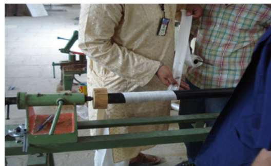
Figure 4.1: Winding of Fiber Tape on PVC Pipe
