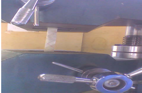
Figure 2.1.1: (a) specimen testing for young's modulus in X-direction
