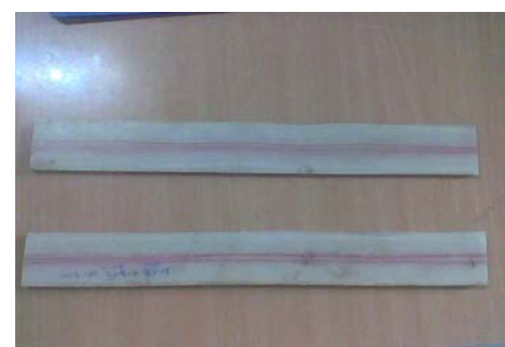
Figure 2.1: (b) Test specimen of orientation [0, 90^\circ]
