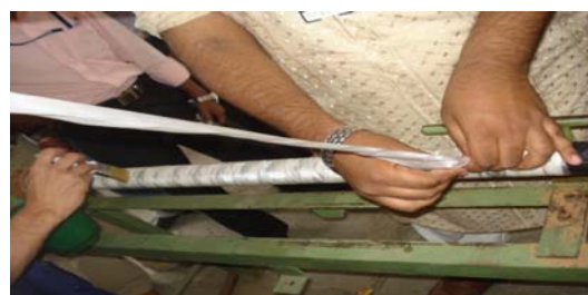
Figure 4.2: Applying of Resin and Winding Tape Simultaneously
