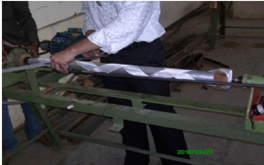
Figure 4.3: Winding of Tape on Aluminum Mandrel
