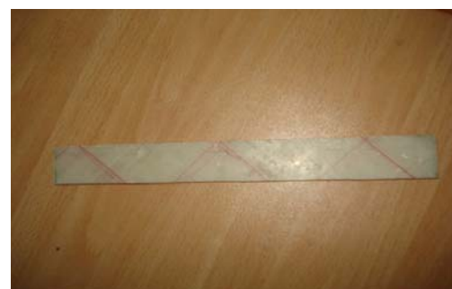
Figure 2.1: (a) Test specimen of orientation [\pm 45^\circ]
