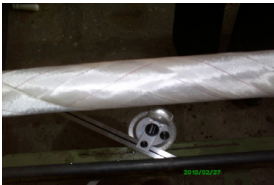
Figure 4.4: First Layer of Tape Winded on Mandrel
