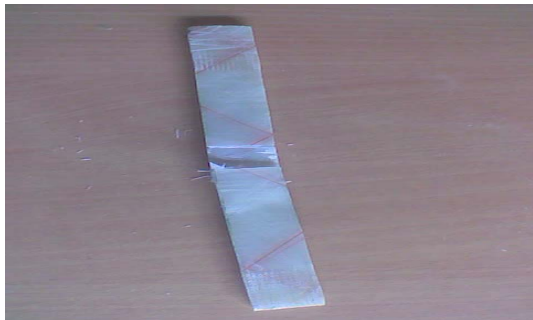
Figure 2.1.1: (b) failure of specimen after test at 45°
