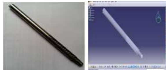
Figure 5: Worm Gear of the Cream Separator and the Catia model developed from it.
