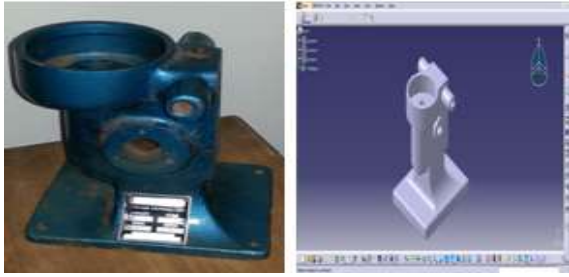
Figure 1: Body of the Cream Separator and the Catia model developed from it.
