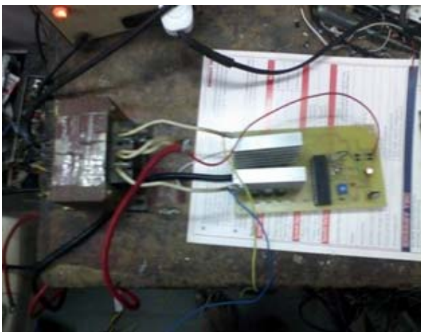
Figure 9: Experimental setup with resistive load bank
