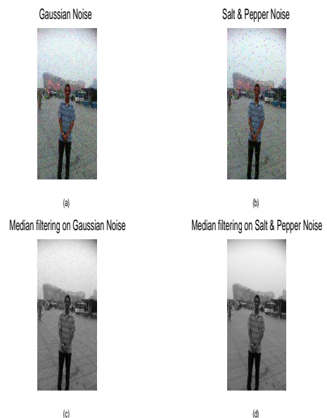
Figure 10: (a) Image corrupted by Gaussian Noise (b) Image corrupted by Salt and Pepper Noise (c) Result of applying median filter on Gaussian Noise (d) Result of applying median filter on Salt and Pepper Noise
