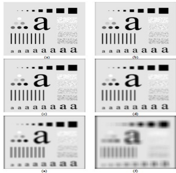
Figure 5: Effect of averaging filters (a) Original Image (b)-(f) Results of smoothing averaging filter mask of size n=3,5,9,15 and 35 respectively.
