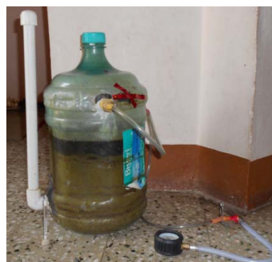
Figure 2: Arrangement of various components of Foliage Gas plant.
