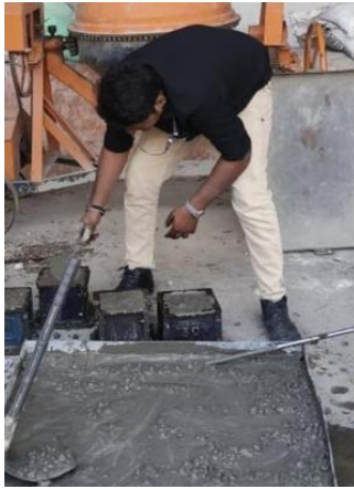
Figure 6: Preparation of concrete cube specimens and testing
