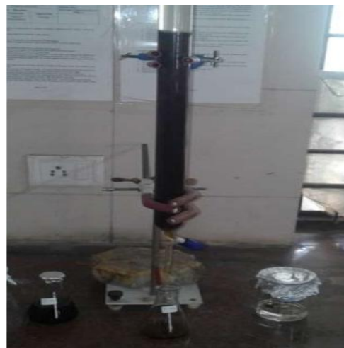
Figure 11: Column chromatography of aqueous layer of ethanolic extract of T. divaricata (leaf Part).
