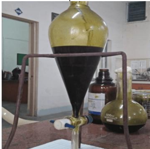
Figure 10: Separating funnel showing separated chemicals in the organic and aqueous phase
