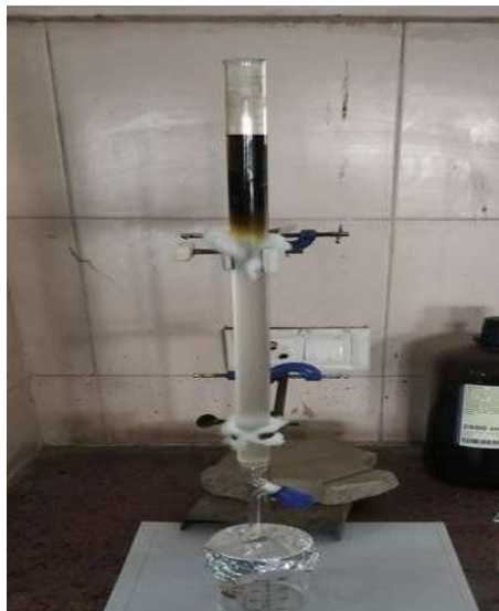
Figure 28: Rechromatography of 5,6th fraction obtained from silica column of aqueous fraction of ethanolic extract of T. divaricata (leaf Part)
