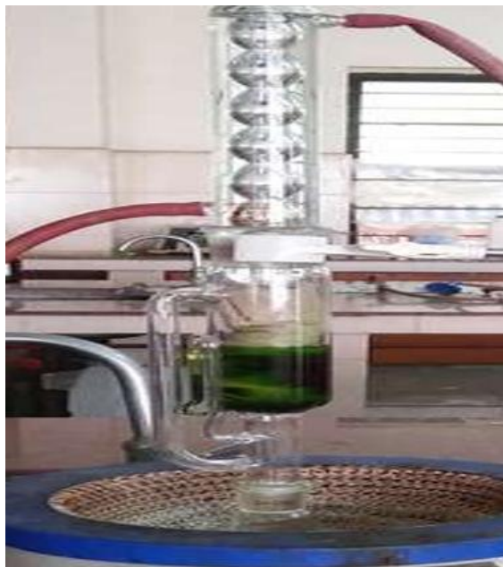
Figure 9: Soxhlet extraction of plant material of T. divaricata
