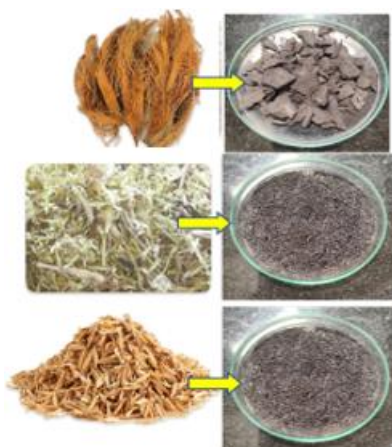
Figure 1: Conversion of agricultural biomass into biochar adsorbents
