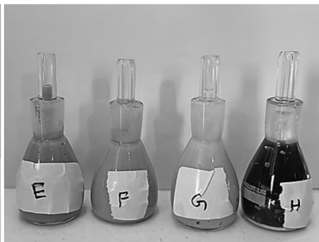
Figure 5 (b): Relative density test for toothpastes (Samples E -H)
