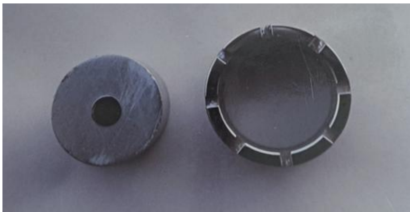
Figure 1: MCT Wafer mounted on jig for Polishing
