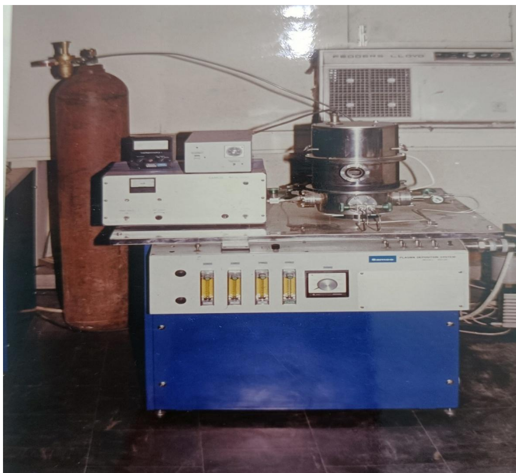
Figure 2: Schematic Plasma Deposition System used for photo-thermal annealing of MCT sample
