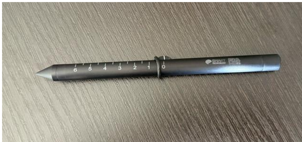
Image 2: Showing the Smart Aesthesiometer with O ring over the device on 0 Position
