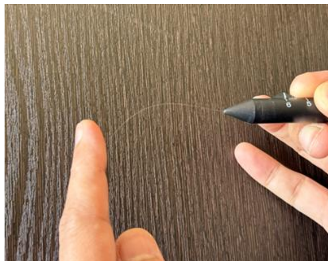
Image 4: Showing the Smart Aesthesiometer with 60 mm Extended filament and showing the force
