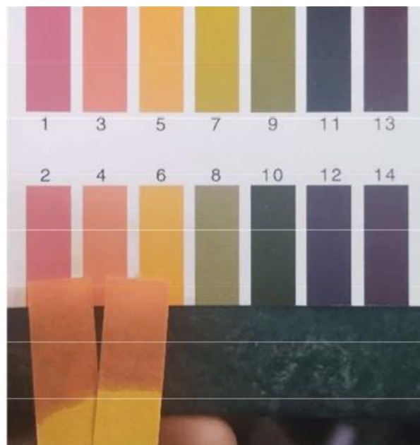
Plates 4.2.9: pH. level 4 - 4.5 of finish
