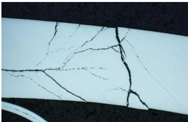
Figure 3: Stress crack in steel surface
