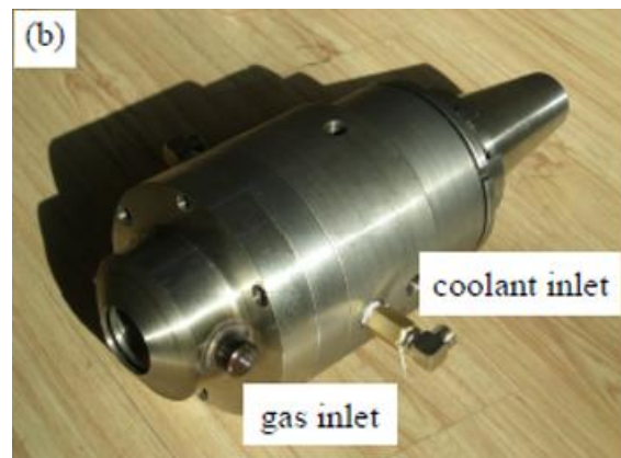
Figure 10: Tool holder with gas inlet (b)
